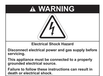
All heater models require constant 120 V 60 Hz 1Ø power supply. Check heater(s) rating plate for electrical rating for proper circuit sizing. For servicing, a disconnect switch of proper electrical rating should be installed in the vicinity of the heater.
